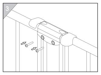
4. Repeat step 3 for the lower panel assembly fitting.
