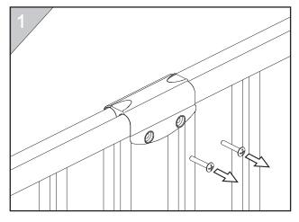
Set the appropriate width of the gate by overlapping the two panels to the extent necessary to allow room for the spindles (parts 10 & 11) on either side of the gate. The maximum allowable overlap is seven bars. The minimum allowable overlap is two bars.
