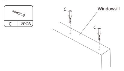
USE ELECTRIC DRILL WITH 1/4"DRILL BIT TO DRILL MARKED 2 HOLES. PINCH ANCHORS TO INSERT INTO HOLES.
