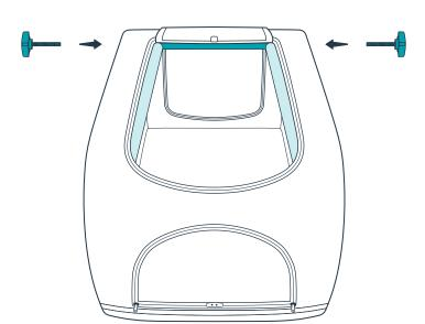
Remove the two star knobs from the ends of the roof support rod. Position the roof support rod inside the trailer, between the top bars of the two side panels.
