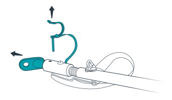
Release the locking pin and remove the black hitch from the tow bar.
