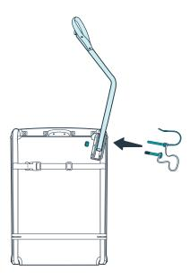
Place the tow bar in the tow bar mounting bracket. Line up the holes at the end of the tow bar with the center holes on the tow bar mounting bracket.
