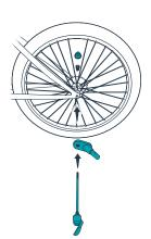
For quick release wheels, remove the quick release skewer from the rear wheel hub, insert it through the hitch, and then reassemble it through the rear wheel hub.
