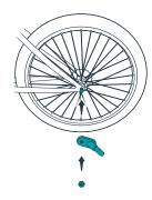
For standard wheels, remove the axle nut, position the hitch on the axle, and reattach the axle nut.
