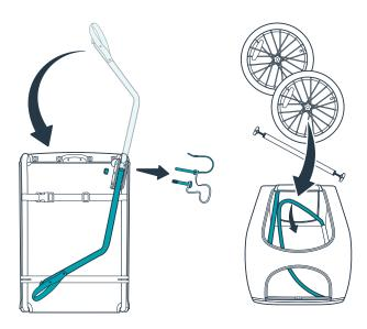
When it's time to store the trailer, remove the locking pin and fold the tow bar under the trailer. Place the roof support rod and wheels inside the trailer, and fold down the side panels.
