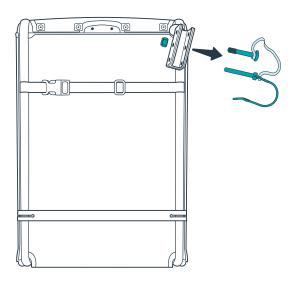
Remove the nut, bolt and locking pin from the tow bar mounting bracket on the bottom of the trailer. Leave the black plastic spacer in place.
