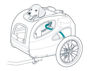
Gently help your dog into the trailer through the rear or top door. Attach the safety tether to your dog's harness and adjust it so it's short enough to keep your dog secure and safe inside the trailer.
