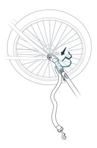
With the trailer behind the bicycle, slide the end of the tow bar over the end of the hitch and secure it with the locking pin.
