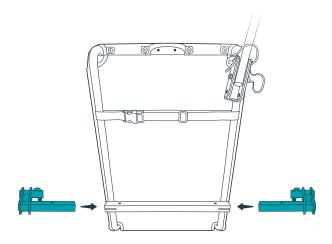
Insert the wheel mounting brackets into the ends of the square brace that runs under the back of the trailer. Make sure the wheel mounting brackets point toward the top of the trailer.
