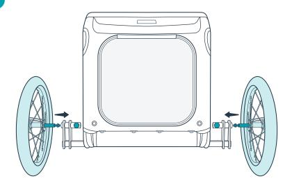
Remove the disposable black plastic cap from each wheel axle. While pressing the wheel lock button, insert each wheel axle into the round hole in the wheel mounting bracket. Release the wheel lock button to lock each wheel in place.
