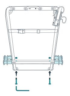
Secure the wheel mounting brackets to the trailer using the nuts, bolts and hex key provided. Use a wrench to hold the nuts while you tighten the bolts.
