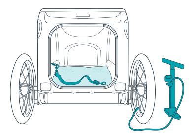
Place the cushion on the floor of the trailer and attach the safety tether to one of the D-rings inside the trailer.
