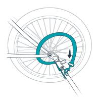
Loop the black safety strap around the bicycle frame and clip it to the D-ring on the tow bar.
