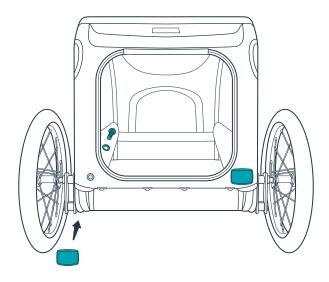
Attach the two reflectors to the back of the trailer by inserting screws and washers through the holes in the fabric shell and into the holes in the back of the reflectors. Tighten with a screwdriver.
