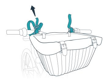
Fasten the safety straps to your handlebars. To make the ride as safe as possible, always be sure these are fully tightened before putting your pet in the basket.
