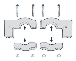
Separate the upper and lower parts of each handlebar mount.
