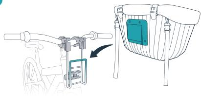
Slide the back pocket on the basket down onto the wire bracket. Check the position and angle of the basket. The curved back portion of the brace should rest firmly against your bicycle's frame.
