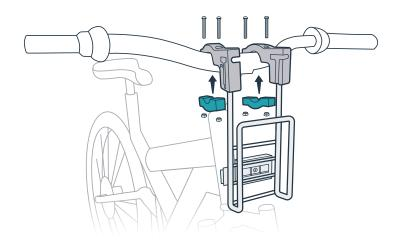
Hang the bracket on the handlebars. (Avoid pinching or bending your bicycle's brake cables.) Reconnect the upper and lower handlebar mounts. You have an extra set of long bolts in case the original bolts are too short for your handlebars.
