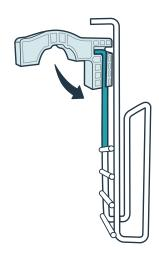
Insert each arm of the wire bracket into the groove on the back of each upper handlebar mount. Rotate each upper mount until the wire stem snaps firmly into the groove. (You'll hear a loud snap.)
