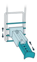
You can adjust the basket's position by extending the brace (move the nut and bolt to any of the five holes) or moving it up or down on the wire bracket. When you're happy with the basket's position, make sure all the nuts and bolts are tight.
