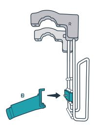
Separate the front plate from the adjustable brace. Position the plate in front of the wire bracket and the brace behind the wire bracket and reconnect them with the nut and bolt.
