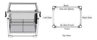
5. Screw the 4 screws firmly onto the metal tubes and then fix the glass lock in the front glass panel.
