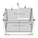
4. When all the four sides have been installed, place the top frame without the top metal ventilation mesh. Make sure that the top frame sits in properly.
