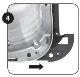
Slide top forward on the base until the front edges are flush.
