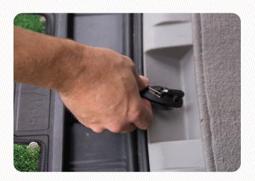
Attach the ramp tether to the rear latch hook of the vehicle when possible. This provides an extra measure of safety. Note, it may not be possible to attach to all makes and models of vehicles.
