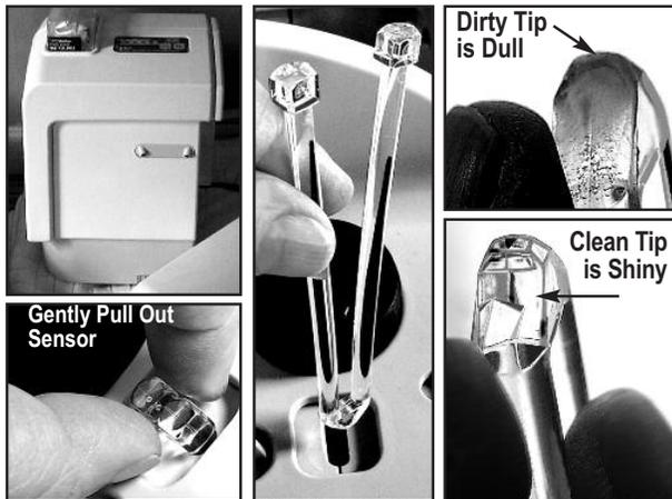
The Water Sensor TIP must be kept free of lime and mineral build up.
