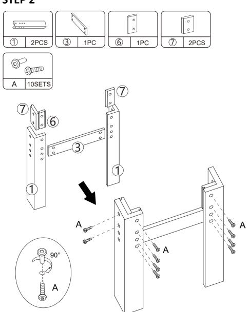
When assembling part ⑥ and ⑦, please do not tighten the screw A.
