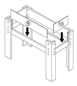
In this step, you can tighten all screw A after inserting two acrylic boards.
