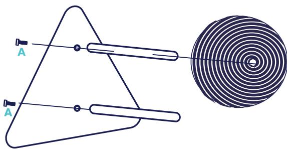
Tighten the 2 screws for easier assembly.
