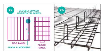
**STEP 2** (a) Locate the side panel without the door and lay it on the floor along the left side of the floor panel. The loops should be facing up. The closely spaced horizontal wires should be closest to the floor panel. (b) Place the floor panel hooks between the second and third horizontal wires and inside the first vertical wires of the side panel.
