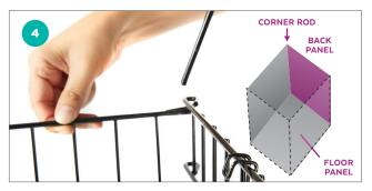
**STEP 4** Locate the back panel and place it at the back of the floor panel and alongside the vertical side panel. The two u-shaped hooks should be on top and facing inward. Align the uppermost loop of the back panel to rest on the uppermost loop of the side panel. Insert the corner rod downward through all of the intersecting loops of this corner.
